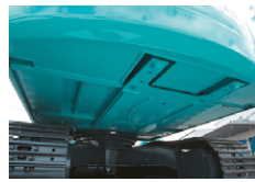
Upper structure undercover
