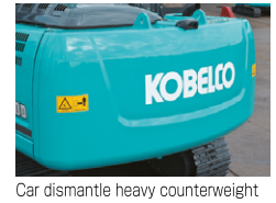
Car dismantle heavy counterweight
